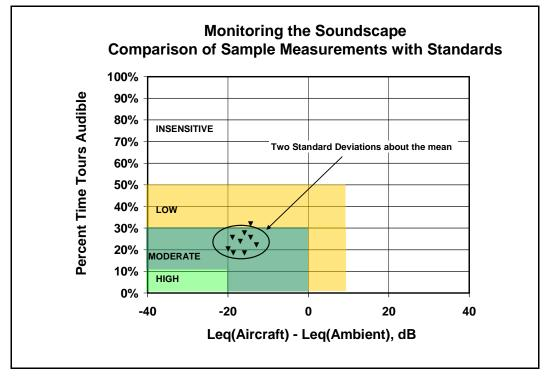
Figure 5 Monitoring results at a location of medium sensitivity to aircraft
