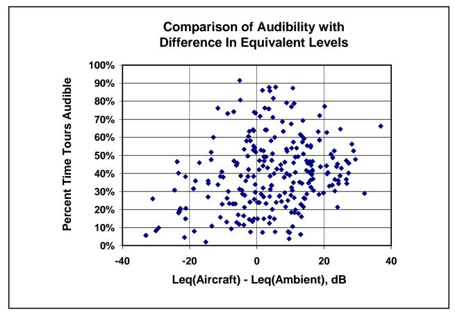
Figure 1 Values of tour aircraft audibility and difference in equivalent levels of 208 measurements
