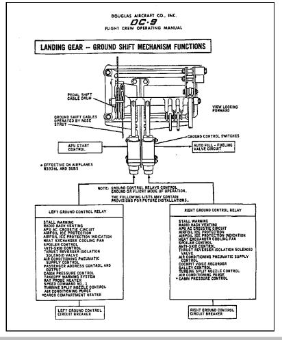
LANDING GEAR -- GROUND SHIFT MECHANISM FUNCTIONS
