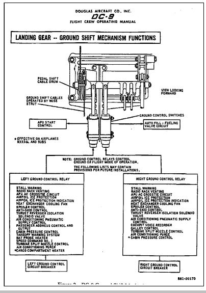
Figure 2--DC-9 Ground Shift Mechanism
