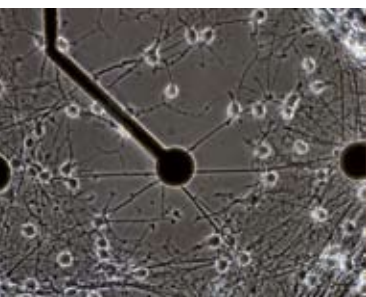
Cortical rat neuron on a micro-electrode array chip.
