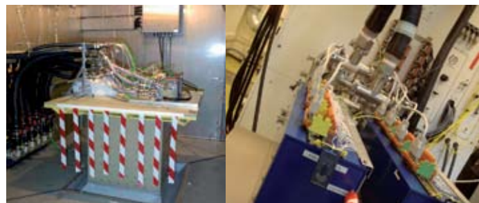
A fuel cell stack undergoing testing in the JRC-IE facility.
