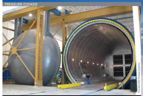
**Biggest baker**: Built to handle the wings and fuselage sections of the 787, this facility at Charleston, South Carolina, is the largest autoclave in the world. The giant pressure cooker operates at up to 232 degrees celsius and 10.2 Bar to "bake" sheets of carbon fibre soaked with resin, turning out solid composite forms.
